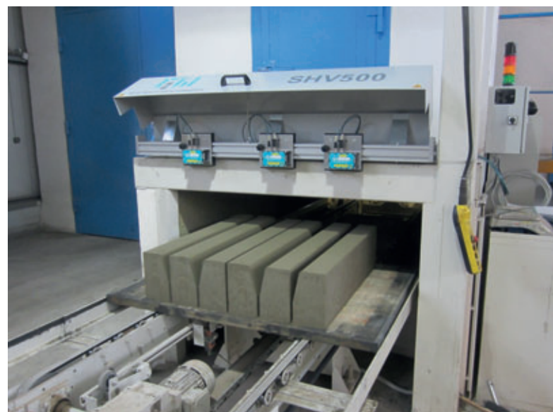
The concrete blocks passing under the device are then measured with the laser sensors without contact and with a precision of +/- 0.5 mm.
